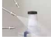
Water Tight Test
