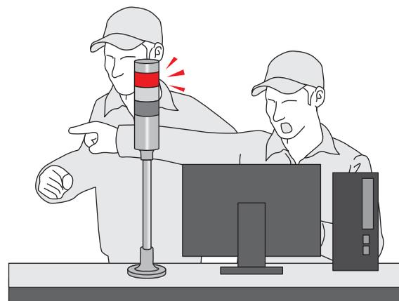
When device abnormalities such as water or dust obstruction is detected, the IO-Link master sends commands to the LR6-IL Signal Tower to activate its visual and audible alarms to indicate the specific problem. Identify device issues before it happens to avoid equipment malfunctions and halts in production.
