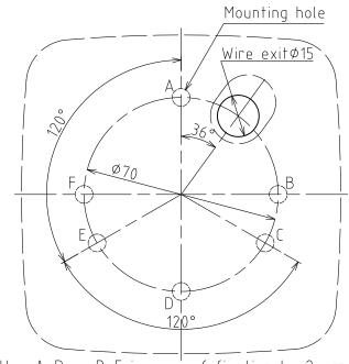
\*Use A-D or B-F in case of fixation by 2 screws. Use A-C-E in case of fixation by 3 screws. And, Install by M6 screw. Mounting surface dimensions
